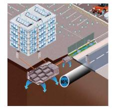
Figure 3: Decentralised infiltration via soak-away structure with infiltration blocks: precipitation water runs into the infiltration structure via channels or pipe drainage or directly from surfaces with infiltration capacity, such as turf. Advantages: less surface area required, less load on the drainage network, the surfaces above the infiltration structure remain usable.
