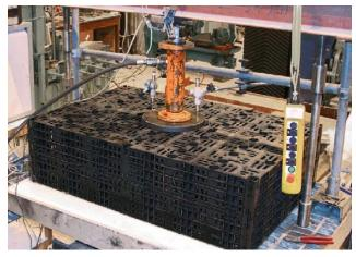
Test with point load from above
